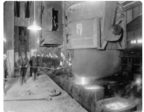
A group of steelworkers at Homestead watch as molten steel is poured into casts.
